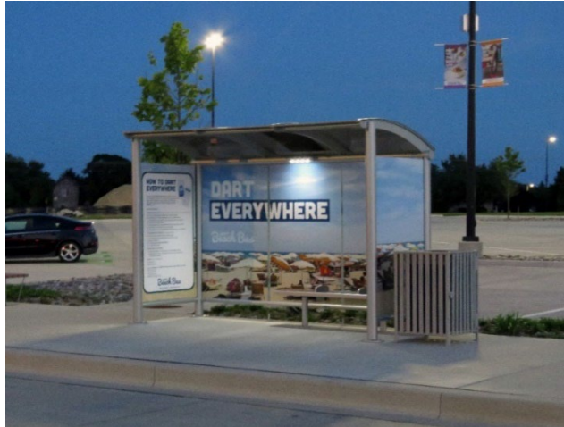
Example of DART's current standard bus shelter
